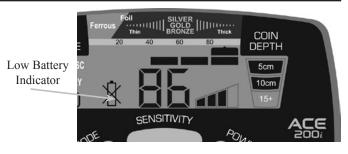
The Low Battery Indicator will switch on when the detector's batteries become weak. The detector will maintain full performance but the batteries should be replaced soon when this indicator appears. NiMH rechargeable batteries may be used, but may have a shorter life per charge. You can expect 20 to 40 hours of operation depending on battery type and quality.
