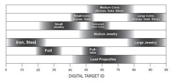
Target ID can vary widely based upon the target's size and thickness because small, thin pieces of metal cannot conduct electrical current as well as thicker pieces of metal. In addition, mineralized soils can cause Target ID errors, especially for small targets.
