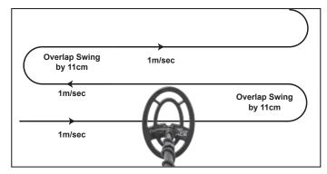
In order to fully search an area, overlap the swings of your searchcoil by half the length of the coil (about 11cm). Sweep the searchcoil in a straight line or with a slight arc at a sweep speed of about 1m/sec.
